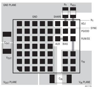
Figure 5. Suggested Power and Ground Planes for LTM8023. Note the Wide Gap that Separates the High Voltage  $V_{\rm IN}$  net From Other Nets, in Compliance with IPC-2221
