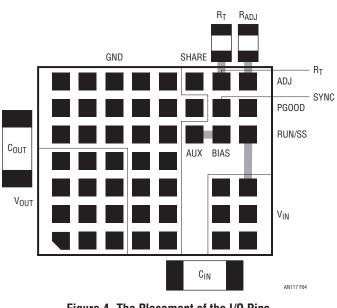
Figure 4. The Placement of the I/O Pins Makes Them Easy to Route.
