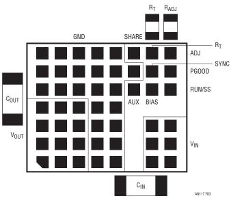
Figure 3. Moving the  $C_{\rm OUT}$  Capacitor Away from  $C_{\rm IN}$  Can Reduce Output Noise
