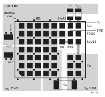
Figure 6. Use Vias to Conduct Electrical Power to Internal Planes and As Heat Pipes to Distribute Heat Throughout the Printed Circuit Board.
