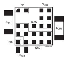
Figure 1. LTM8020 Example Component Placement
