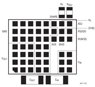
Figure 2. LTM8023 Example Component Placement
